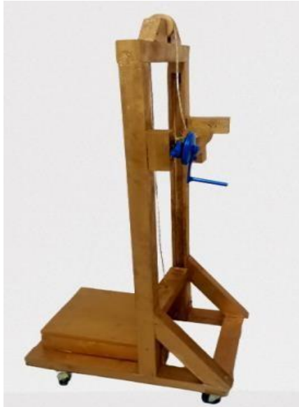
Gambar 4. Prototype Lift Manual Pengangkatan Larutan Emulsifier
