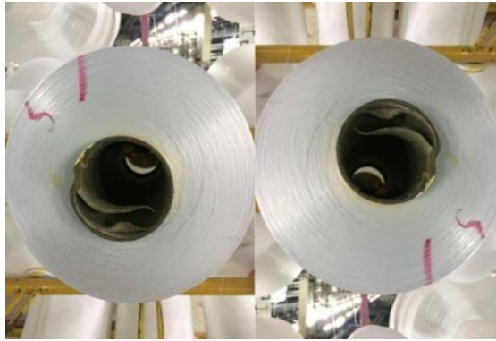
Gambar 9 Damaged Paper Tube
