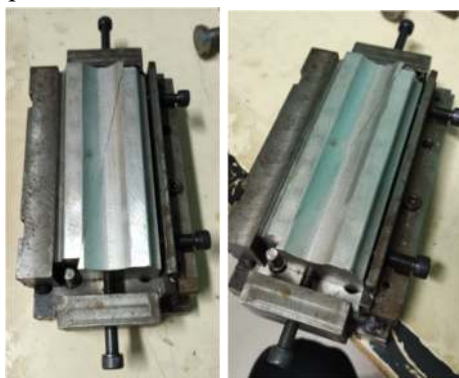
Gambar 1.2 Fixture Bantalan Sling (Sumber : Pribadi)
